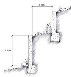
Retaining walls, where required by grade, shall be a maximum of six (6) feet in height measured from the lowest Natural Grade (measured on the outside of the wall). If multiple walls are required to retain a grade there shall be a six (6) foot minimum separation as measured from the back of the lower wall to the front of the upper wall suitable for planting landscape material; provided, however, the ARC may permit alternative wall designs for Lots with extreme elevation changes.
