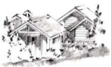
Massing is the arrangement of three-dimensional building solids that form the exterior of the home. Each Residential Unit must be composed of multiple masses with each mass distinguished by a vertical and horizontal offset.
